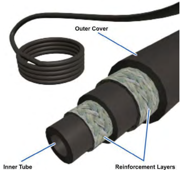
Figure 9-49 — Flexible rubber hose construction.
